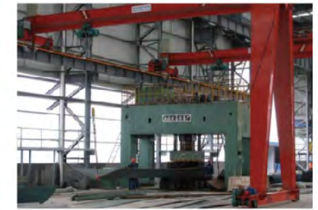
1000T油压机 1000T hydraulic machine
