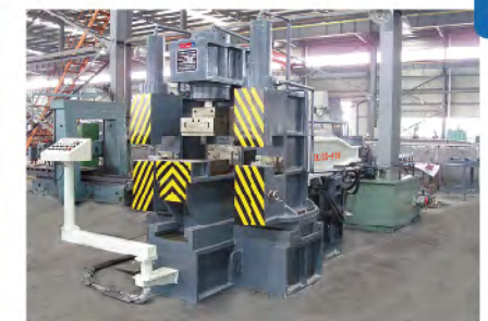
400T 肋骨冷弯机 400T frame bending machine
