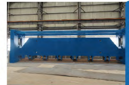
12.5m三辊卷板机 12.5m three-roller plate bender
